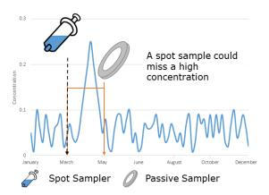
To reduce the non-representativeness of spot sampling, passive sampling techniques are an option. Passive sampling relies on the unassisted molecular diffusion of pesticides through a diffusive barrier onto an adsorbent surface over a prolonged period of deployment. These samplers are designed to maximize the mass of pesticide accumulated in order to detect the generally low levels of pesticide present in water.
