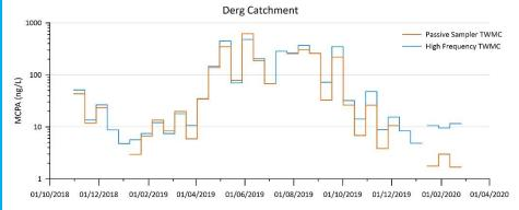
Time-weighted mean concentrations determined by both techniques were comparable across a range of timeweighted average concentrations (the Y axis is on a log scale) for this combination of pesticide and hydrologically flashy river.
